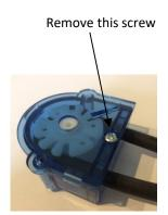
Squeeze tubes together and lift out rotor. If tube is fitted with blue "C" clips leave in place on tube. Rotate the rotor complete with tube so the other drive size is towards you.
