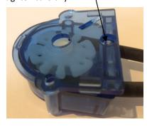
To refit the pump head first carefully locate "D" on motor shaft into the "D" in the rotor. Rotate pump head until mounting holes line up with holes in bracket. Remove pump & place mounting screws through pump head. Fit rubber washer on screw threads so that they will end up between pump head & bracket. Refit pump head and do up screws carefully. Screws must tightened sufficiently to partially compress rubber washer not completely flatten them.
