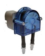
The 200 series, range of peristaltic pumps offer a low cost, compact & reliable means of dosing a wide range of liquids. They are available in various configurations of tubing type & size giving flow rates of between 0.1 & 1.32 ml/rev. The pump head is designed to be disposable but is assembled using a single screw enabling dis-assembly & re-assembly for tube changing if required.
