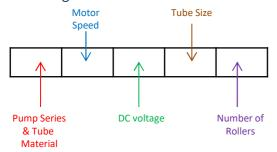
202-035-024-016/4 Example product code for 200 series pump head fitted with Viton® tubing , 35 RPM, 24v DC, 1.6mm ID tubing & 4 rollers
